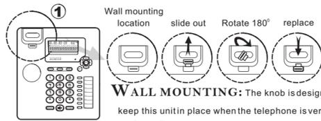
**WALL MOUNTING:** The knob is designed to keep this unit in place when the telephone is vertical on the wall.
